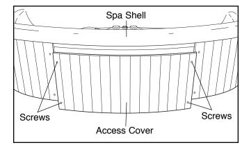
If the spa will be stored for any period of time, place the power cord inside the spa unit before re-attaching the access cover.
